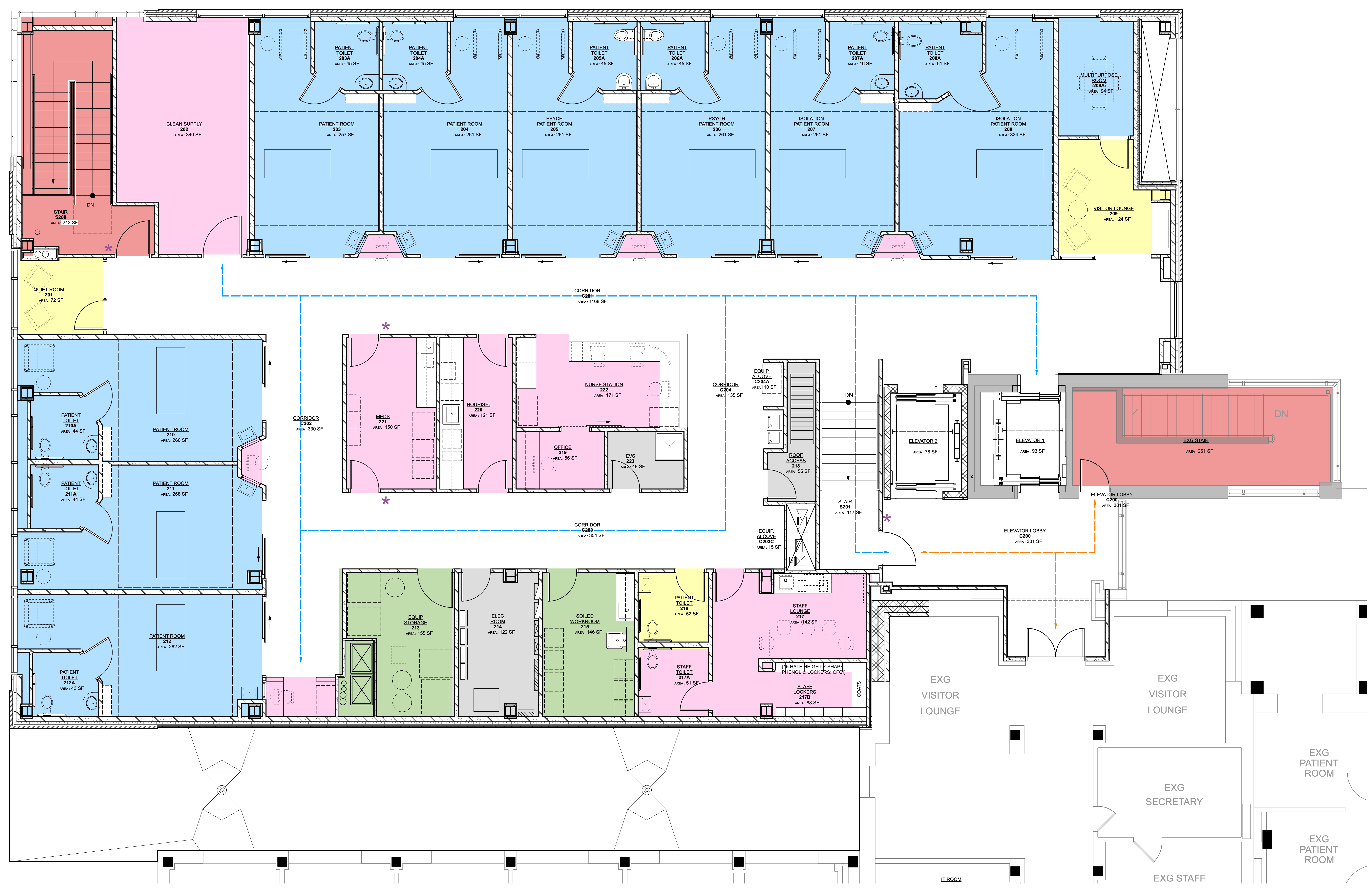
B1 CIRCULATION PLAN - SECOND FLOOR Scale: 1/4" = 1'-0"
